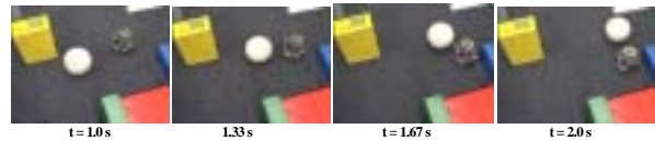
Fig.8 Avoidance (0.5 s) of Mobile Robot 2004 against an approaching high speed ball during searching for Red color.
