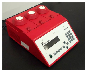
3. Advanced multicycler (T3 thermocycler, Biometra) DNA amplification and reaction of DNA sequencing
