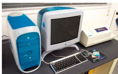
5. Microplate Spectrofluorometer (SPACTRAMax GEMINI, Molecular Devices) Measurement of fluorescence of multi sample
