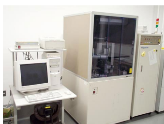
X-ray diffractometer (RIGAKU R-AXIS RAPID)
