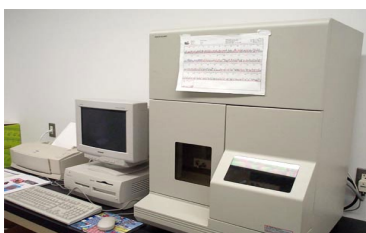
4. Genetic Analyzer (ABI PRISM 310, ABI), Determination of DNA sequences
